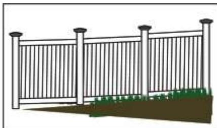
The tongue-and-groove privacy panels allow for a minimal amount of racking. The maximum level of racking for these panels is 3/4" per 8' panel. To accommodate uneven terrain, it may be necessary to cut each picket to "fit" the slope.
